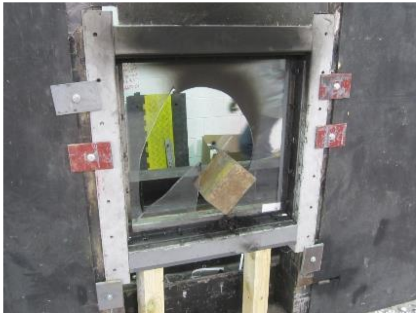
Photo No. 6 Specimen No. 2 - Body Passage Failure
