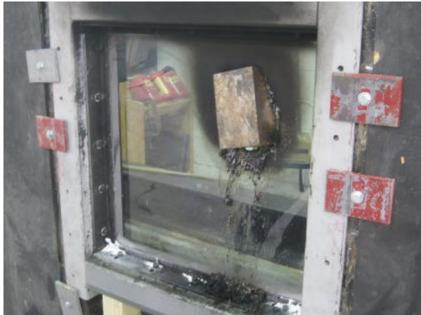
Photo No. 3 Specimen No. 1 - Body Passage Failure
