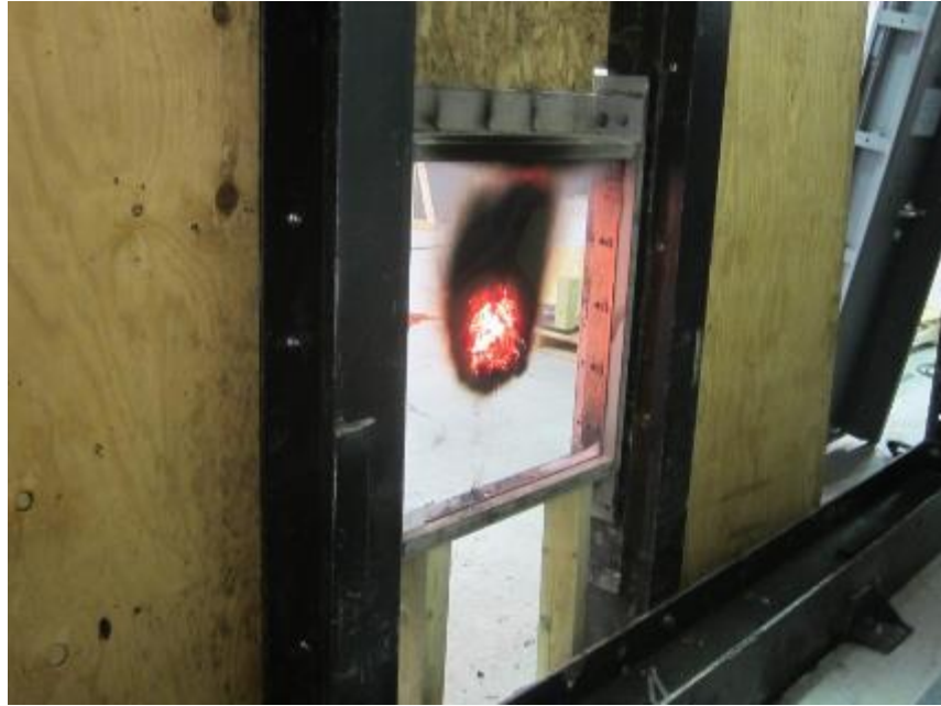
Photo No. 5 Specimen No. 2 - Contraband Failure
